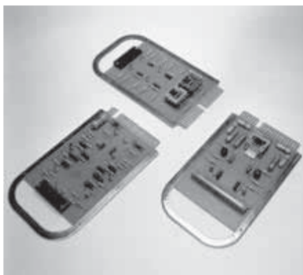
Cartes prototypes DTL (Photo FT/R&D)
